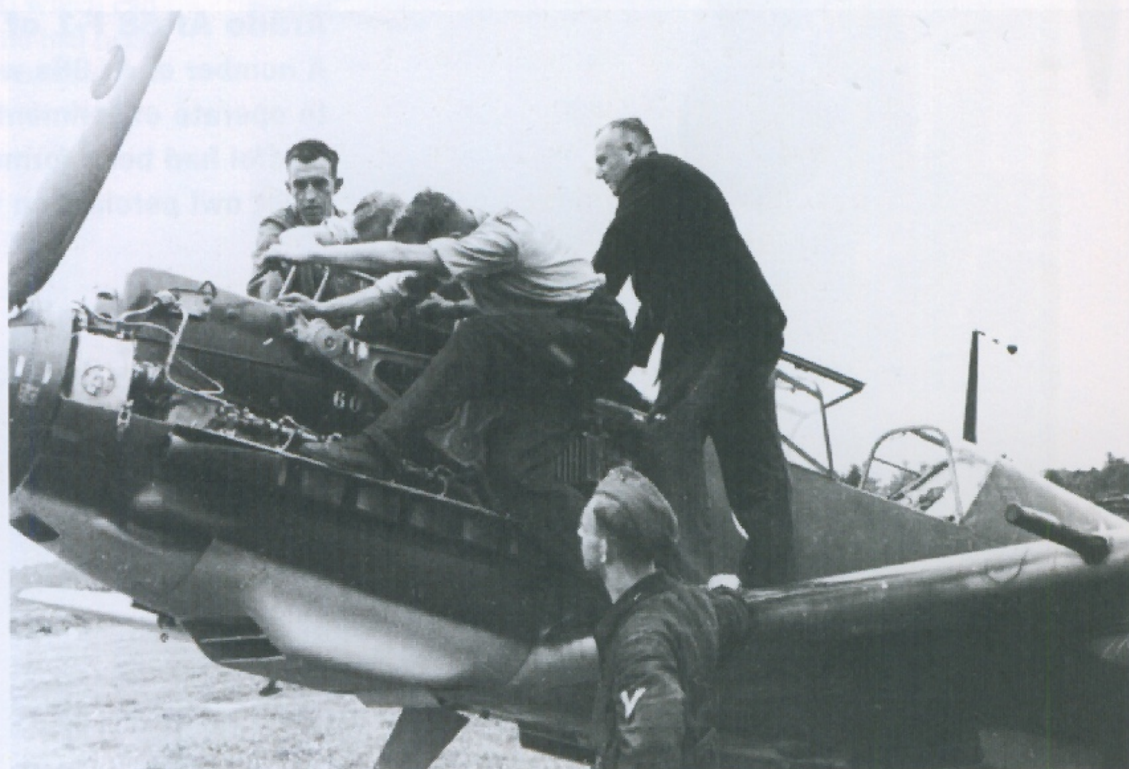
ABOVE: Mechanics at work on the Daimler-Benz DB 601 A engine of a Bf 109 E-3. The aircraft carries a segmented upper surface camouflage pattern of black-green (RLM 70) dark green (RLM 71), standard for the early months of the Second World War, with pale blue (RLM 65) underneath.
