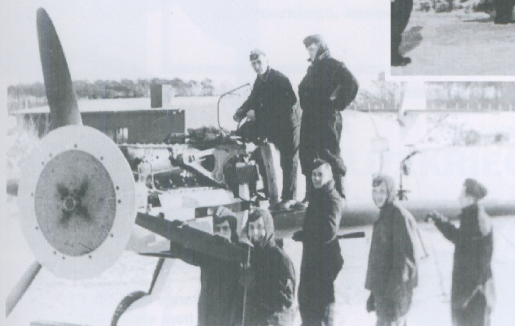
ABOVE AND LEFT: Taken at Mannheim-Sandhofen in the snow of winter 1939/1940, this Bf 109 E coded 'Red 1' of 6./JG 52 is having its machine-guns synchronised. The aircraft may have been flown by the Staffelfkapitän, Lt. Werner Lederer. It is interesting to note that the Staffel's aircraft now have light blue (RLM 65) fuselage sides with the top of the fuselage and wing upper surfaces camouflaged in a splinter pattern of dark-green (RLM 71) and RLM grey (RLM 02).
