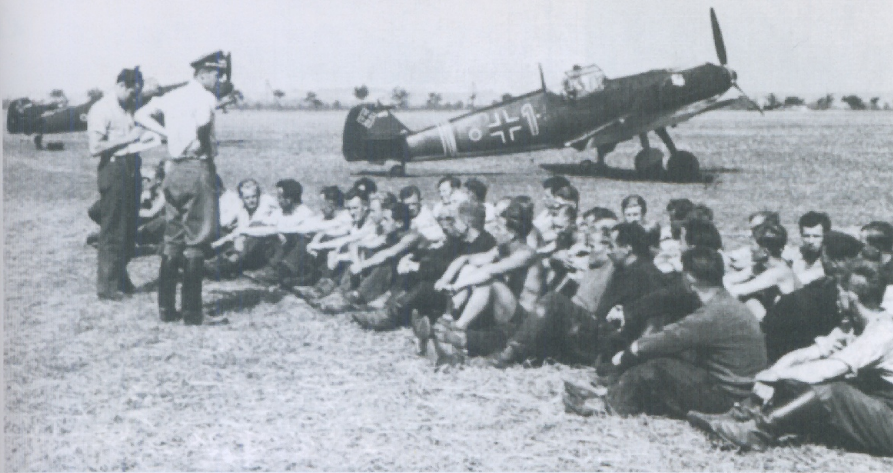
LEFT: Hptm. Hannes Trautloft, (standing with hands on hips) with the men of 2./JG 77 during the Polish campaign. The Bf 109 E in the background 'Red 1' was painted black-green (RLM 70) on the upper surfaces with light blue (RLM 65) underneath. The aircraft also has a red circle outlined in white and three white fuselage bands. The one nearest the front appears to be double the width of the other two. These markings may have been used as identity markings during training and manoeuvres. The gun ports have also been painted yellow, not an uncommon practice, as was the spinner.
