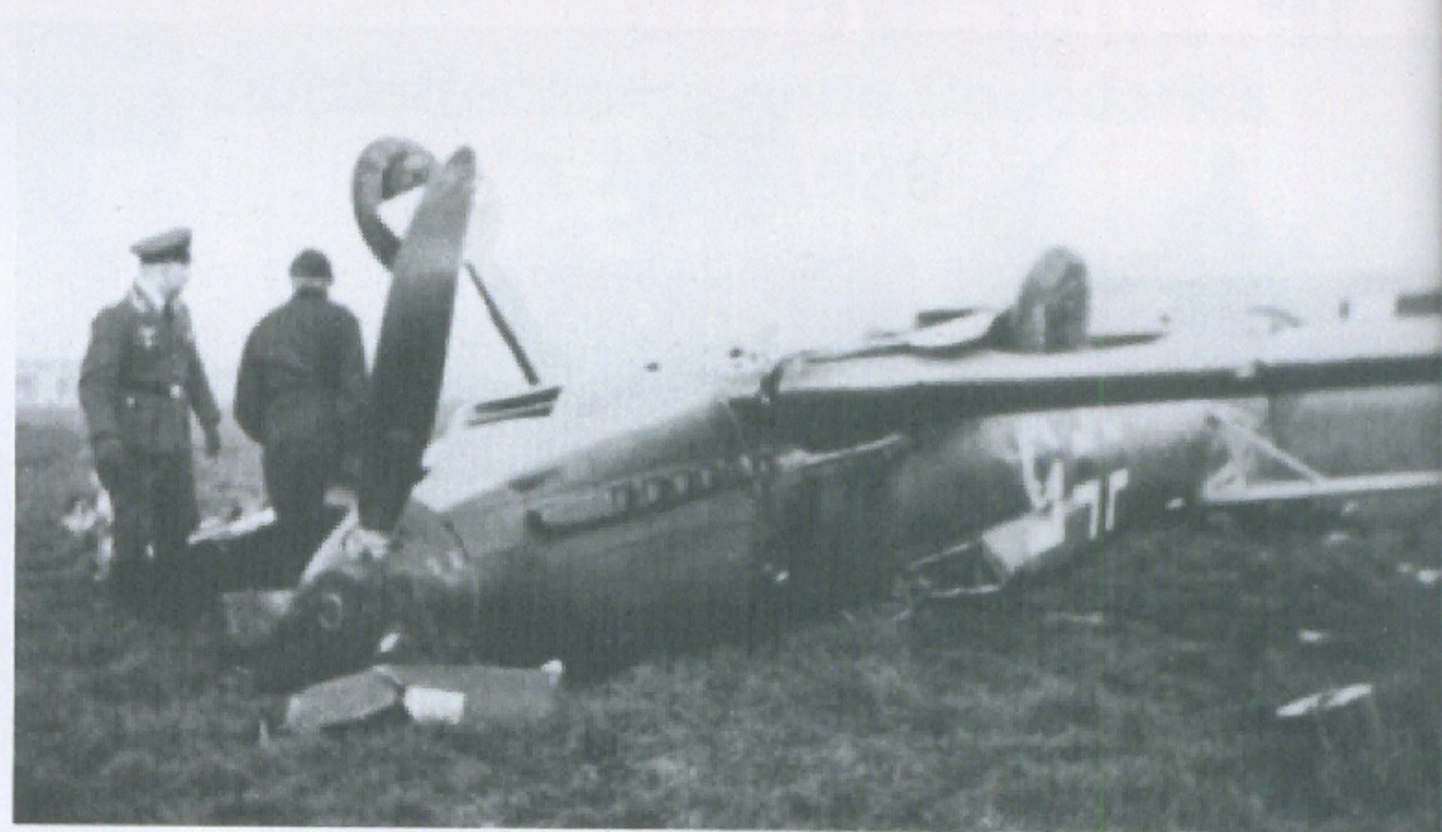
ABOVE: Accidents were not uncommon with the Bf 109 E. Here 'White 5' of I./JG 51 has flipped over on to its back at Bad Aibling following the collapse of its starboard undercarriage leg during a landing in the spring of 1939. Note the black-green (RLM 70) and light-blue (RLM 65) demarcation line running to the leading edge of the wing compared to the photo on the left.
