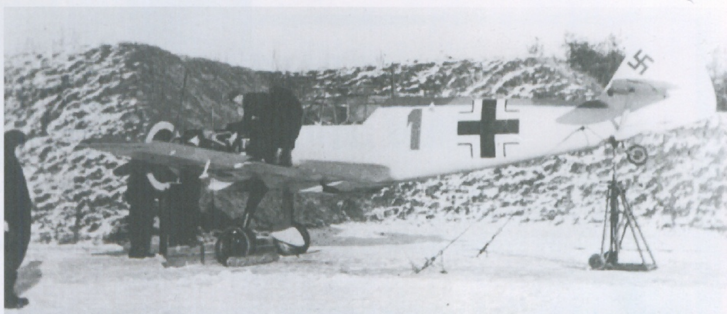
ABOVE AND LEFT: Taken at Mannheim-Sandhofen in the snow of winter 1939/1940, this Bf 109 E coded 'Red 1' of 6./JG 52 is having its machine-guns synchronised. The aircraft may have been flown by the Staffelfkapitän, Lt. Werner Lederer. It is interesting to note that the Staffel's aircraft now have light blue (RLM 65) fuselage sides with the top of the fuselage and wing upper surfaces camouflaged in a splinter pattern of dark-green (RLM 71) and RLM grey (RLM 02).
