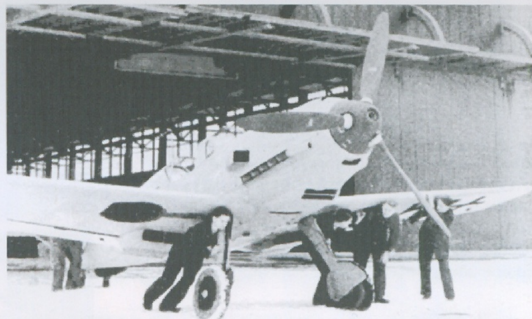
ABOVE: A brand new Bf 109 E-1 is pushed out into the snow from the assembly hall. The aircraft still carries its radio call sign and is painted light blue (RLM 65) all over except for the spinner and propeller which have the standard finish of black green (RLM 70).
