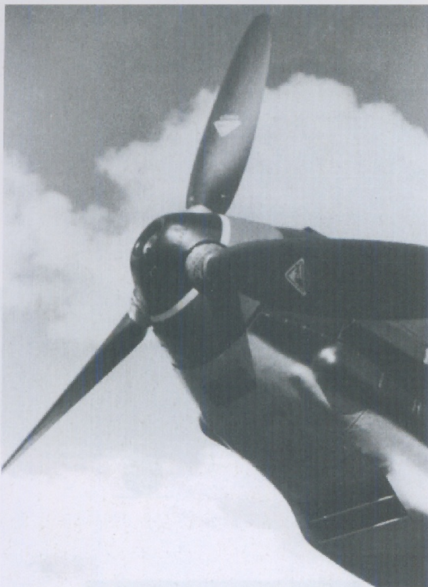
LEFT: The spinner of this Bf 109 E from 2./JG 1 had a black-green (RLM 70) nose with a narrow white ring and red hub. The propeller was also painted black-green and had the VDM logo on the front of each blade.
